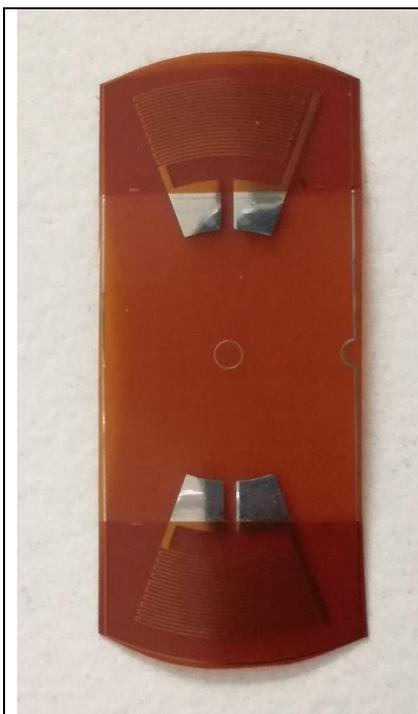
Figura 53. strain gauge
