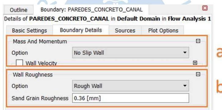
**Figura 102.** Boundary details de la frontera *PAREDES\_CONCRETO\_CANAL*.
