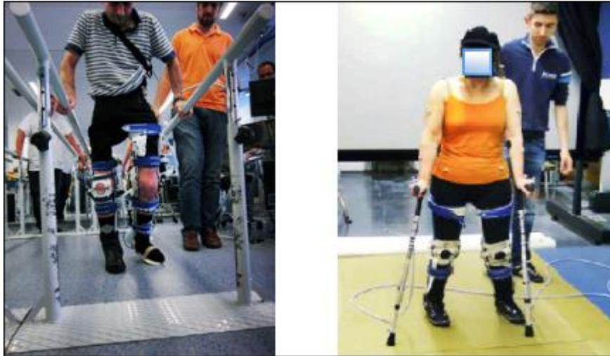
*Figura 52 Prototipo de la órtesis usada en diferentes pacientes. (Fuente: Lugris, U. et al. (2013). Gait Analysis System for Spinal Cord Injured Subjects Assisted by Active Orthoses and Crutches)*
