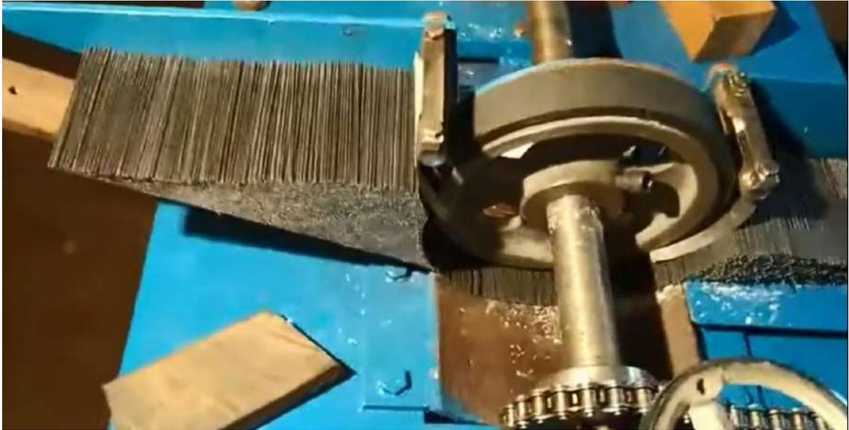
Fuente: Steel tip grinding machine - part 2 of fishing hook production line, por CHINA DLC MACHINERY CO., LIMITED (s.f.), YouTube
