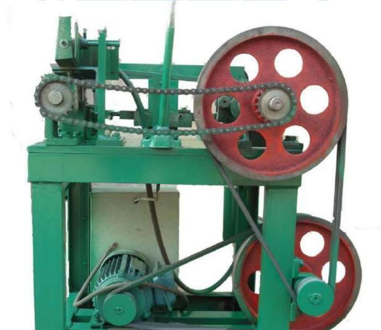
Fuente: Bending Machine for Squid Hook, por Quzhou Waterford Fishing Tackle Co., Ltd (s.f.)
