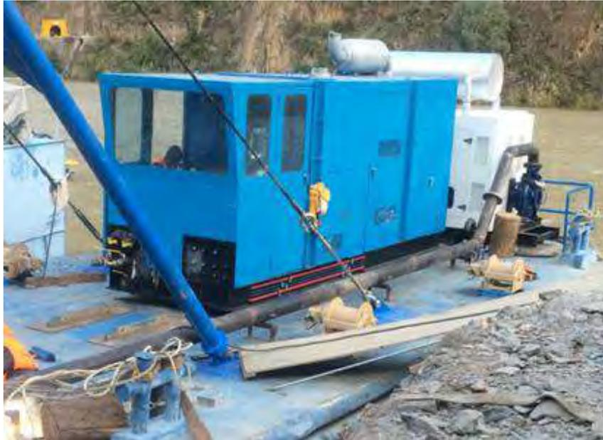
**Figura 88.** Motor power pack de 570 HP.
