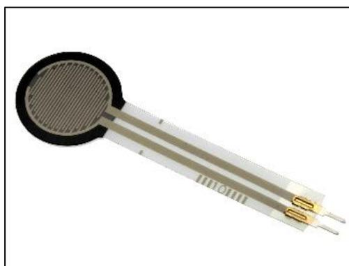
**Figura 30:** *Force Sensor Resistor.*
