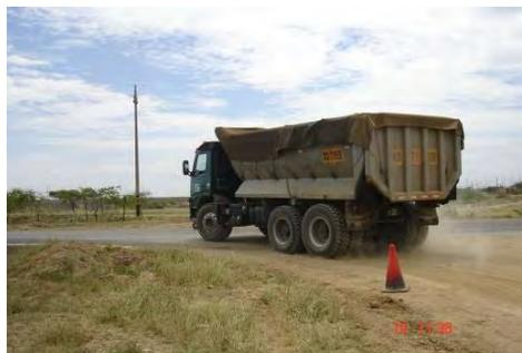
**VOLQUETE DE 16 m<sup>3</sup> PARA EL TRANSPORTE DE LA MEZCLA ASFALTICA**
