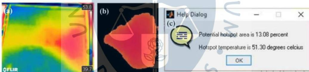
Tomado de “Hotspots Detection in Photovoltaic Modules Using Infrared Thermography” (Salazar & Macabebe, 2016).
