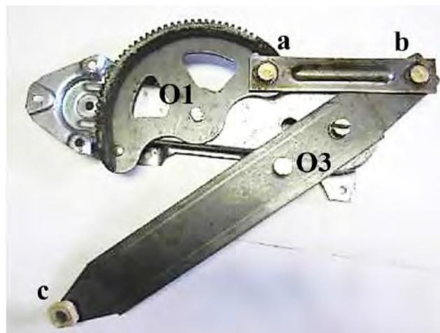
**Figura 117.** (1984-1994) Ford Tempo Topaz Front Driver's Side Power Window Regulator W/O Motor
