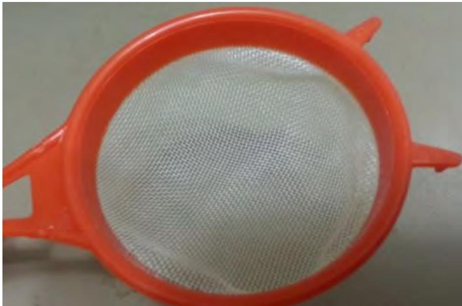
**Figura 39.** Tamiz #30 ASTM (600  $\mu\text{m}$ )
