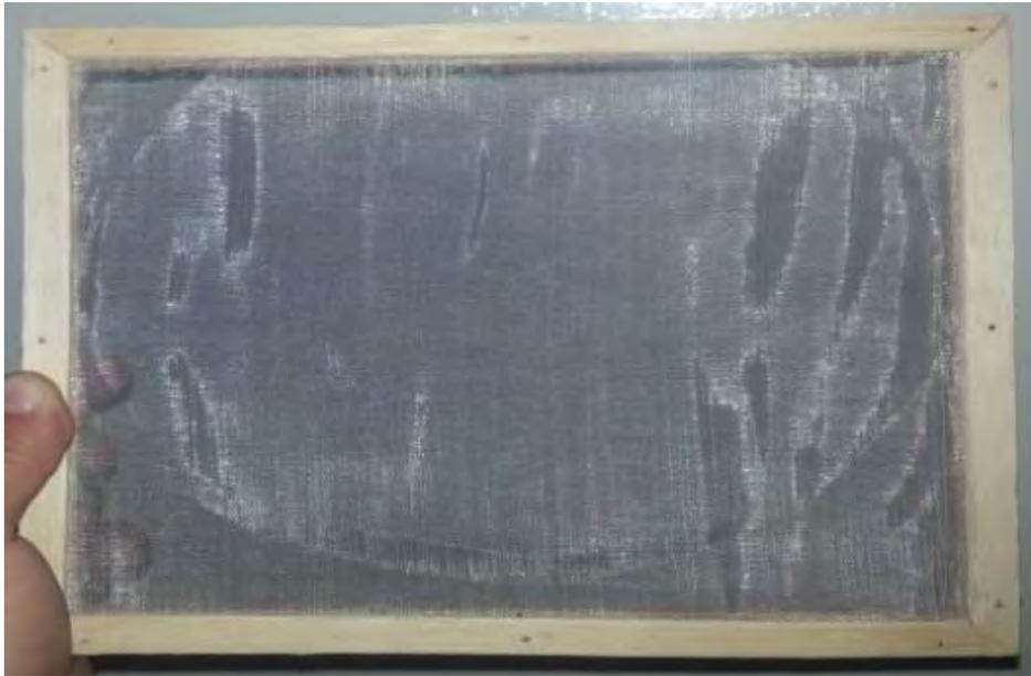
**Figura 38.** Tamiz #60 ASTM (250  $\mu\text{m}$ )
