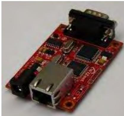
Fig. 4.51 Circuito RS232 – Ethernet
