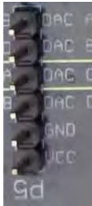
**Fig. C.9** Conector del DAC
