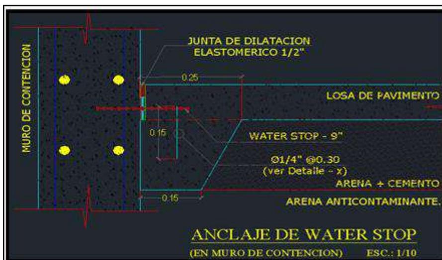
**Figura 6.** Anclaje de water stop.
