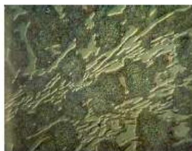
Figure 2, Typical Microstructure of 28G Alloy (Magnification 400X)
