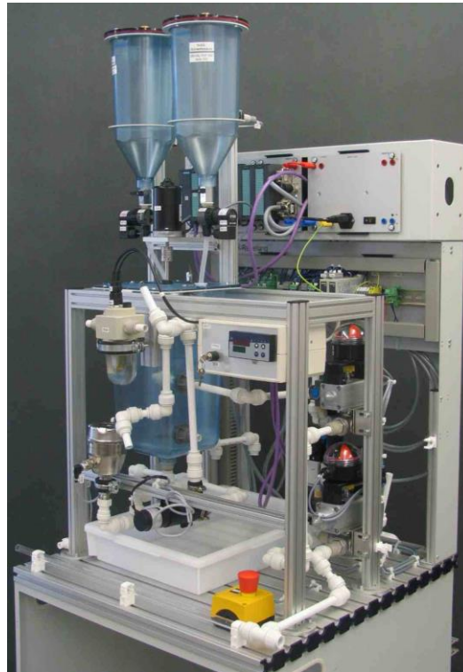
Figura 9 - Planta piloto pH Workstation FESTO Didactic
